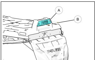
2. Remove rear cargo platform © by removing ten screws ①.
