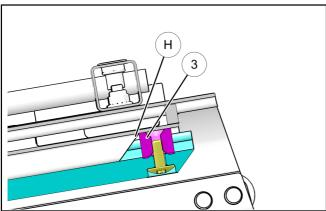
6. After installing wear strips, replace the close off/ snow flap assembly © using provided fasteners @ and ⑤ as shown. Torque fasteners to specifications listed.
