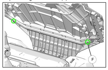
9. Place front rack extender assembly on front rack (B) and install two screws (5) and nuts (6). Do not tighten fasteners.
