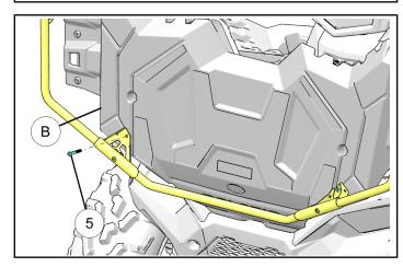
10. Close the front rack (B) along with rack extender assembly. Reinstall two screws (A) removed in Step 4 on front rack (B) through rack extender assembly as shown.
