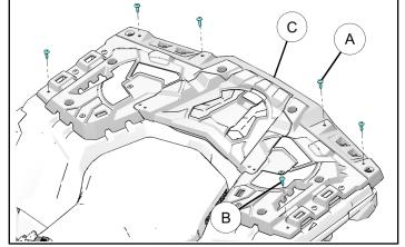
Install rear rack extender assembly on rear rack as shown and install four screws (A) removed in Step 3 to the rectangular rear rack extender ①. Tighten fasteners to specification.
