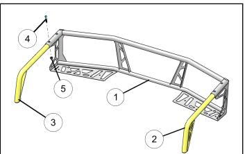
5. Reinstall two screws (B) removed in Step 3 onto the rear rack extenders (LH 2 and RH 3) from the bottom side of the vehicle as shown. Tighten fasteners to specification.
