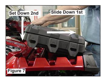
8. Lower the rear of the box and make sure it fits flat on the front of the vehicle.
