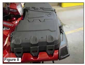
9. Verify that the box is properly installed. **NOTE:** The front of the box must be secure in the front rack support, check this by trying to lift up on the front of the box. If the box comes loose, repeat the process starting from Step 6.
