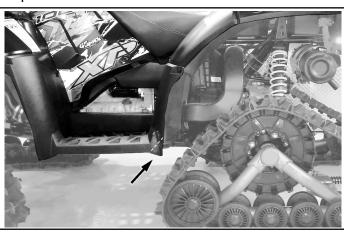
Measurement (A) is approximately 60mm (2.36") and measurement is approximately 100mm (3.93")
