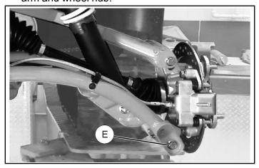
6. Position anchor bracket ® under lower suspension arm. Slip C-shaped end of bracket on suspension arm cross-member.
