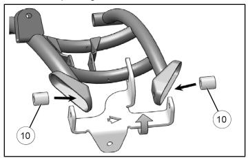
8. Insert M10x200 mm bolt ① through anchor bracket, spacer bushings, suspension arm and steering knuckle. Use the flange nut ⑪ provided to assemble the parts together. Torque nut to specification provided.
