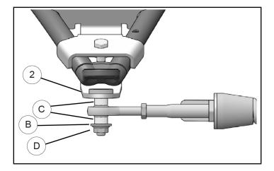
4. Position steering limiter cable assembly under front anchor bracket. Use the provided bolt (6), washer (9) and nut (20) to secure the assembly in the center of the anchor bracket as shown. Torque to specification provided.
