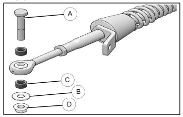
5. Remove bolt © securing the lower suspension arm to the wheel hub. A new M10-1.5x200 mm bolt (provided in the mount kit) will be used to assemble the anchor bracket, lower suspension arm and wheel hub.
