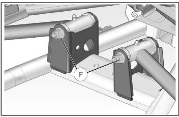
2. Install the suspension stiffener plate on the lower a–arms mounting bolts. Secure the stiffener plate using the nylon nuts provided. Torque nuts to specification provided.
