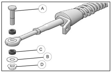
5. Insert the bolt (A) in the front anchor bracket (2)/(3) as shown.
