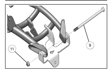
9. Secure the undercarriage to the rear hub using the nuts ② provided in this mount kit.
