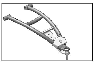
10. Secure the undercarriage to the front hub using the nuts ② provided in this mount kit.
