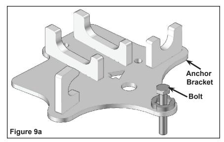
5. Position anchor bracket under the lower suspension arm; C-shaped openings on bracket must fit suspension arm tubing. Figure 10 and Figure 10a.
