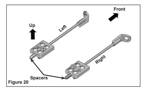
On each FRONT track system, position the bended extremity of steering limiter on stabilizing rod between hex grip and rubber damper washer. Figure 21.
