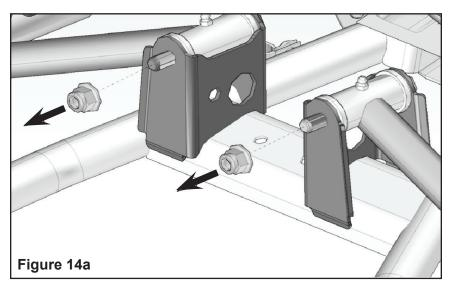
Insert the suspension stiffener plate on the lower a–arms mounting bolts. Secure the stiffener plate using the nylon nuts provided. Torque the nuts to 37 ft. lbs. (50 Nm). Figure 15 and Figure 15a.
