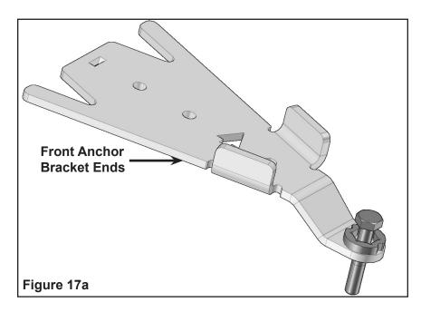
Position the bottom part of the anchor bracket underneath the lower suspension arm. Position the top part over the suspension arm so the tab slips in the slot in the bottom part. Insert the M10x50 mm bolts through the bottom and secure the two parts together with the nuts provided. Tighten assembly to 37 ft. lbs. (50 Nm) of torque. Figure 18 and Figure 18a.
