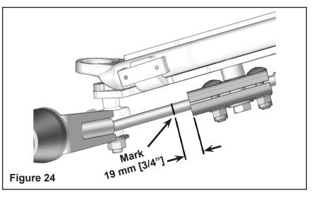
Align the mark on the cable and the edge of the clamping blocks. In a criss-cross sequence, tighten to 18 ft. lbs. (25 Nm) the four hex nuts. Figure 25.
