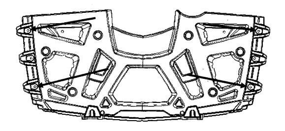
3. Drill out the front holes for the rack extender bolts shown below. Drill from the bottom side. There should already be holes through the aluminum tubing, use them as a pilot.
