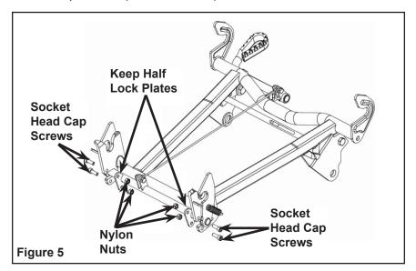
7. Fasten the hook up extension and extension plates using four M6-1 x 25 mm socket head cap screws, four M6-1 x 18 mm socket head cap screws and eight M6-1.0 hex. Nylon nuts. Figure 6.
