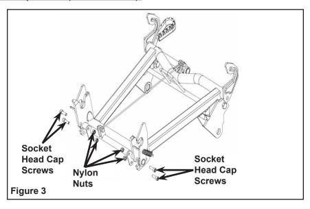
7. Fasten the hook up extension and extension plates using four M6-1 x 25 mm socket head cap screws, four M6-1 x 18 mm socket head cap screws and eight M6-1.0 hex. Nylon nuts. Figure 4.
