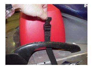
3. Cinch buckle down to the grab handle. It is important that the buckle is pulled tight to the bar. This ensure the buckle will be located properly.
