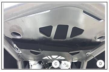
5. Secure the bag ① with two rear Velcro straps (C) around rear rack tubes as shown.
