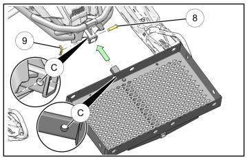
b. Ensure hitchpin clip (9) is fully seated into the groove on the clevis pin (8) as shown.
