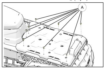
Place Titan Rear Rack ① onto rear platform, align mounting holes and fasten with the eight screws
