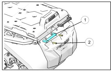
2. Start both bolts (2) by hand and torque to specification.
