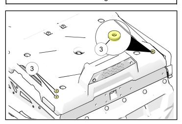
3. Place the Titan Tail Light Protector into position and place one washer ③ on top of the Titan Tail Light Protector ① over the mounting holes as shown.
