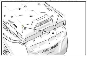
2. Place two of the supplied washers ③ on to the Titan Rear Cargo Platform over the mounting holes as shown.
