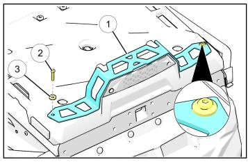
Secure in place using the provided screws ②. Torque to specification.
