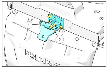
2. Insert the four screws ② supplied with your kit and torque to below specification.
