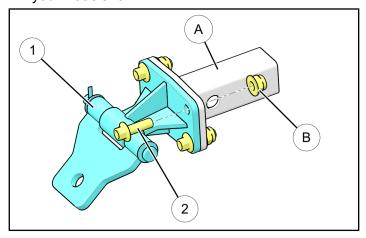
2. Secure the two assemblies together using the four locking nuts ® that were supplied with your Titan Adapter Hitch Kit, PN 2882814, A and torque to the listed specification.
