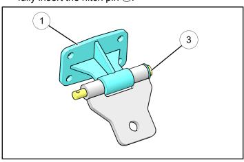
3. Place remaining washer ④ on the end of the hitch pin ③ and secure in place by inserting the supplied cotter pin ⑤ in the pre-drilled hole on the end of the hitch pin. Use a needle nosed pliers to bend over the tabs of the cotter pin to secure it in place.
