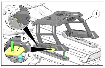
Once the front of the passenger seat support is fully seated, lift the latching mechanism handles Dupwards and firmly press down on the back of the passenger seat support until the latching mechanism is fully engaged onto the latching pins (E).
