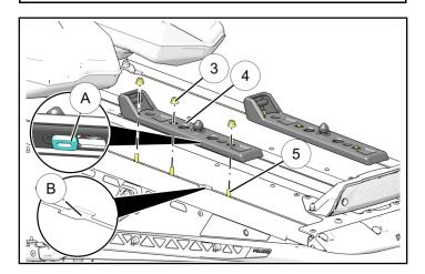
4. After placing both tunnel latch plates into the proper position, start all six locking nuts ③ by hand. Torque to specification.
