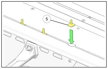
3. Next, align the three mounting screws (5) up with the mounting holes in the tunnel latch plate (4) and place the tunnel latch plate into position as shown. Repeat for opposite side.
