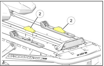
To remove the covers, use a flat screwdriver or similar tool to gently pry up on the outer edge of the cove until it is no longer seated in the mounting holes.
