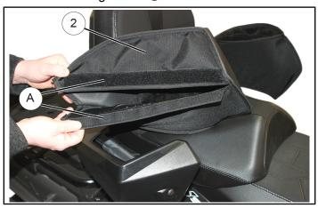
3. Place gauntlet ② over the top of the passenger hand hold ® as shown.
