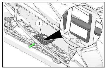
2. Install the right hand lower mounting brackets ③ using the supplied fasteners ⑤. Start all fasteners by hand then torque to specification provided.
